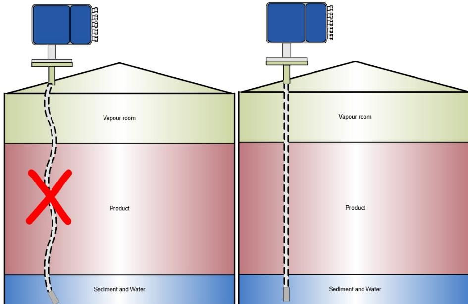
The counterweight should not touch the bottom of the tank to let the probe hang straight in the tank. The temperatures measured by a Pt100 in the probe should represent the average temperature of the whole area at the height of the Pt100. The ambient temperature might have too much influence when the probe is mounted close to the tank side.
