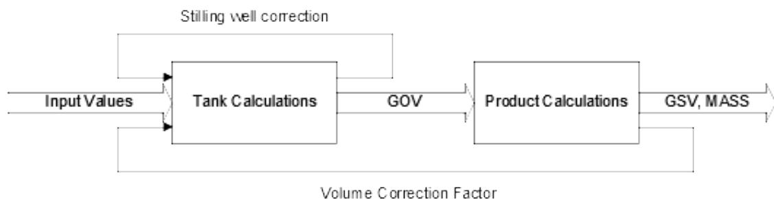
Levels are corrected for stilling well expansion due to temperature. Average temperatures are used to calculate the corrections. Average temperatures are calculated using the corrected level. This explains the iterative stilling well loop in the drawing above. The Volume Correction Factor (VCF) is a result of the product calculations and it is used in the tank calculations to calculate a floating roof correction when required.
