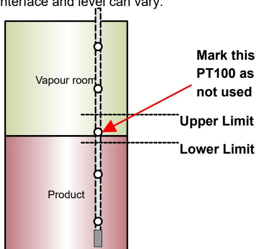
Linear weight factors are calculated by the height of the layers and used for stilling well and shell expansion correction purposes. Volume weighted averages are calculated by the volume of the layers and are used for volume correction factors. (VCF)
