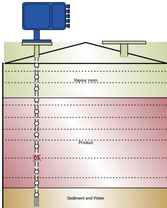
A Multipoint temperature probe is used to measure the average temperatures with the highest achievable accuracy. A tank contains typically 3 compartments, sediment and water, stored product and vapour room. Up to 16 temperature spots can be measured. The locations of the Pt100's in the probe can be tailored to customer needs.
