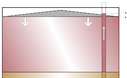
According to Archimedes law the weight of the replace liquid compared to the level in the stilling well is the same as the weight of the roof.
