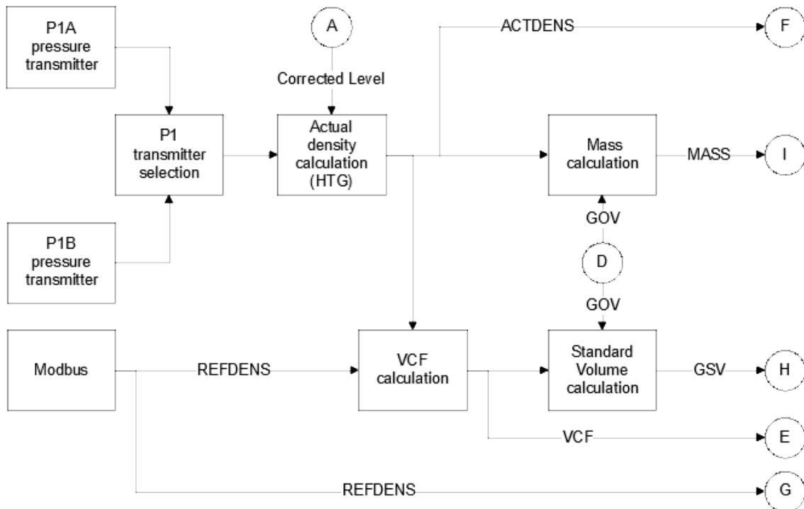
In many cases pressure readings are not available. Either reference density or actual density must be available to calculate the volume under reference conditions and the mass. It is most likely that a reference density is made available via Modbus. The next diagram shows the calculation for this case.
